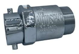
3" (76mm) Male NPT x 2.5" (65mm) Female swivel hose thread, polished chrome Check Snoot. The HF325M CP is used on multiple inlet fire department connections, enabling the connection of several fire department supply lines at one time. The HF325M CP is equipped with a brass clapper preventing the backflow of water through unused connections. A breakable cap or plug should be installed to protect swivels, and reduce the risk of foreign debris from entering the connection. UL/ULC Listed.
