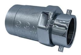
3" (76mm) Female NPT x 2.5" (64mm) Female swivel hose thread, polished chrome Check Snoot. The HF325F CP is used on multiple inlet fire department connections, enabling the connection of several fire department supply lines at one time. The HF325F CP is equipped with a brass clapper preventing the backflow of water through unused connections. A breakable cap or plug should be installed to protect swivels, and reduce the risk of foreign debris from entering the connection. UL/ULC Listed.
