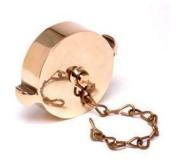
2.5" (DN 65) threaded brass cap & chain for protection of male outlet threads on valves and hydrants. Also, prevents entry of foreign material. Specify regional hose thread.
