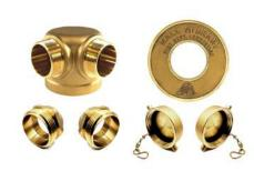
4" (100mm) NPT x 2.5" (65mm) hose thread x 2.5" (65mm) hose thread, brass angle free-standing wall hydrant used as an auxilliary water supply by the fire service. The body is furnished with two F x M brass adapters to create 2.5" (65mm) hose thread outlets. The package also includes two caps and chains, a round "Wall Hydrant" escutcheon plate. Option for 18" polished brass sleeve. The IE36-WH BR provides 250 GPM per outlet. Specify regional hose thread. UL listed.
