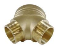
4" (100mm) NPT x 2.5" (65mm) NPT x 2.5" (65mm) NPT brass straight roof manifold used as a standpipe roof outlet connection, fire pump test connection or wall hydrant by the fire service professions. The body is furnished with female NPT inlet and male NPT outlets. The IE35 provides 250 GPM per outlet. UL Listed.
