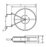
A= 37.5" (953mm) B= 31" (787mm) C= 9" (229mm) D= 13" (330mm) Reel=26"(660mm) F= 13.25 (337mm) G= 2" (50.8mm)
