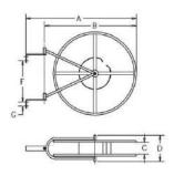
A= 34" (864mm) B= 30" (762mm) C= 5.5" (140mm) D= 9.5" (241mm) Reel=26"(660mm) F= 13" (330mm) G= 2" (50.8mm)
