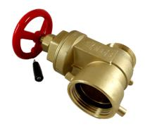
2.5" Straight Pattern Brass Gate Valve with non-rising stem and swivel inlet. For use on hydrants, standpipes and fire pump test connections rated for up to 300 lbs (2070 kPa) applications. The IE27W is made up of a brass body and brass trim and comes with a red round handle, and optional speed handle. Rocker lugs or pin lugs are available on the inlet swivel and male hose thread on the outlet. Specify hose thread.
