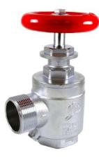
300 lbs (2068 kPa) pressure tested approved valve. Heavy Duty 1-1/2" (38 mm) chrome angle hose and hydrolator valve. Automatically drains and vents, safeguarding against hose deterioration. O-ring packing and red cast handle. Forgeline Bonnett and Seat Assembly. UL/ULC listed and FM Approved. Specify NPSH or NST thread for outlet.
