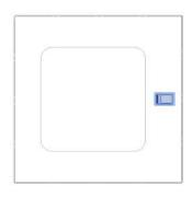
14" (356mm) x 14" (356mm) x 8" (203mm) Surface style valve cabinet constructed in 16 gauge Cold Rolled Steel. Interior and exterior are treated with our exclusive WILCO "**PRO-TECH**" *Premiere* prime coating system. The door is fitted with 3/16" (5mm) clear glass, stainless steel concealed latch and reinforced piano hinges.
