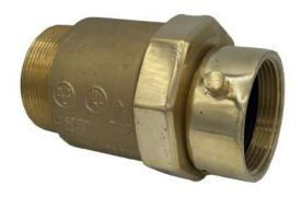
3" (76mm) Male NPT x 2.5" (65mm) Female swivel hose thread, polished brass Check Snoot. The HF325M is used on multiple inlet fire department connections, enabling the connection of several fire department supply lines at one time. The HF325M is equipped with a brass clapper preventing the backflow of water through unused connections. A breakable cap or plug should be installed to protect swivels, and reduce the risk of foreign debris from entering the connection. UL/ULC Listed.
