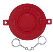
2.5" (65mm) inexpensive molded red plastic protective plug for swivel connections. The quick plug has breakable ears, where two eye bolts and nuts are for attachment to female pin or rocker lug swivel. The quick plug prevents entry of foreign materials and can be easily removed with a fire department spanner wrench.
