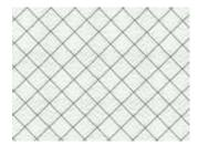
6 mm (1/4") thick 38" (965mm) x 10" (254mm) Georgian Polish Wire glass for the IE11CV type extinguisher/valve cabinets. The GPW glass is a double pane glass with a Georgian Polish Wire in the middle that holds most of the glass if broken. The GPW glass is a stronger pane of glass then the standard glass and will withstand a greater impact. The glass is used primarily in complexes where risk for breakage may occur.
