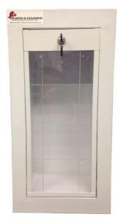
8.5" (216mm) x 19.9" (506mm) x 6.3" (160mm), inside dimensions, recessed mounted extinguisher cabinet constructed of 22 gauge steel. Cabinet is featured with quality cylinder lock, glossy white powder-coated enamel finish for corrosion protection, easy glass removal for extinguisher servicing and is readily installed. Cabinet does not include the breaker bar & chain.
