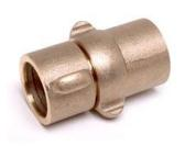
1 1/2" (38mm) Forged Brass coupling with brass expansion ring, a swivel washer and tail washers. The coupling comes with rocker lugs on the female and male ends and is used on collapsible rack & reel hose. Specify regional hose thread.
